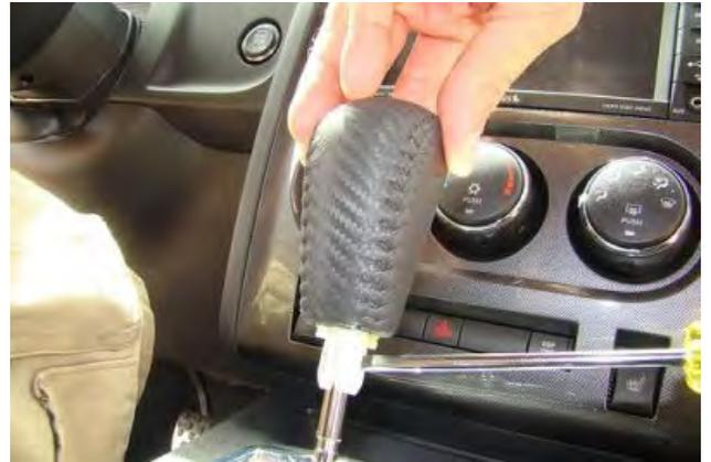
3. **Friction Snap** – With a small flat-tip screwdriver, carefully spread the locking fingers apart while pulling the shifter handle upward, until the handle comes free.
