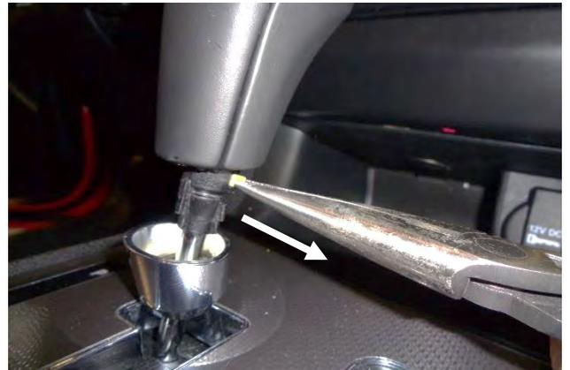
4. **Spring Clip** – Use pliers to pull the spring clip out of the shifter handle, then lift the handle off the shifter stick.
