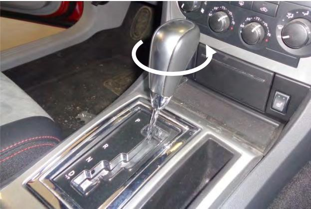
1. **Threaded** – Threaded shifter handles simply twist off the shifter stick in a counterclockwise direction.
