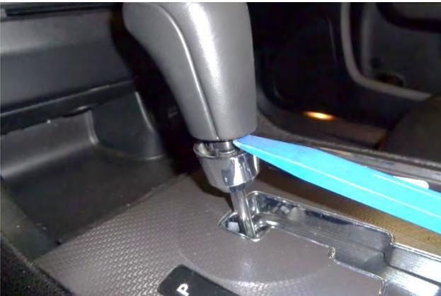
2. **If your shifter handle is not threaded**, carefully pry the chrome trim ring off the shifter handle. This will reveal the how your handle is attached. NOTE: Do not pry the trim ring off threaded shifter handles!
