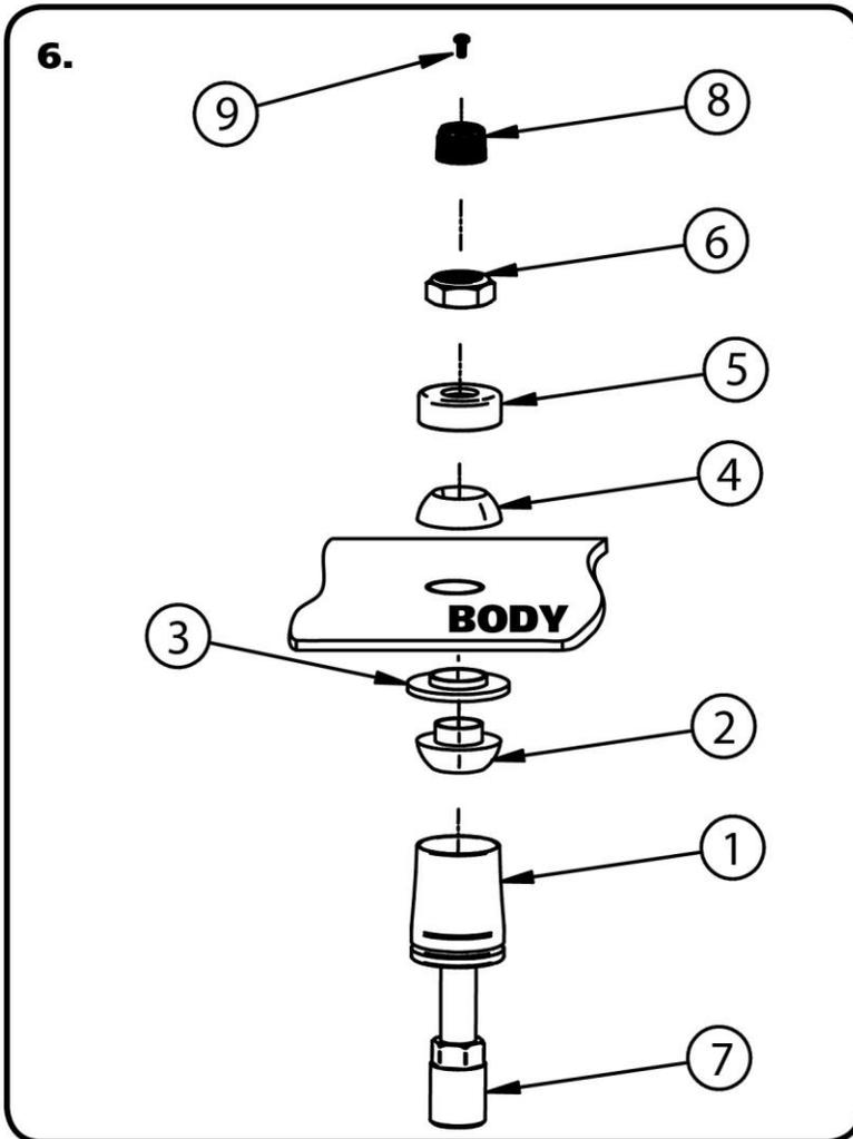
6. The air fitting location can be rotated by twisting the bellow assembly separate of the shock. Place the Shockwave into the OEM shock location with the stud sticking through the OEM shock hole. See assembly **Diagram 6**.
