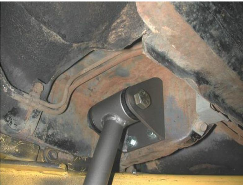
9. Bolt the new front lower bar mount to the body using 4  $\frac{3}{8}$ " x  $1\frac{1}{4}$ " bolts, 8 flat washers and 4 Nyloc nuts.
