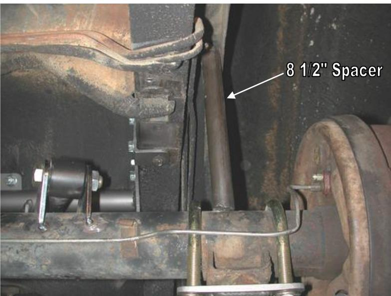
11. Before welding the tabs to the axle pinion angle must be set; the axle must be centered between the rails; and the axle must be raised to ride height. One trick to help maintain these setting is to tack weld a **temporary**  $8\frac{1}{2}$ " spacer between the body and the axle.
