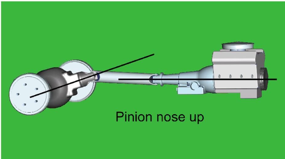
12. How do you set the pinion angle? On a single-piece shaft you want to set it up where a line drawn through the center of the engine crankshaft or output shaft of the transmission and a line drawn through the center of the pinion are parallel to each other but not the same line.
