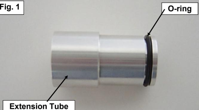
Place the extension tube on the transmission filter (**See Figure 2**).
