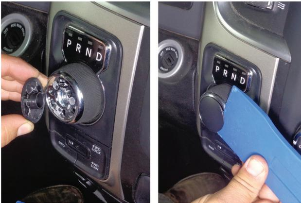
2. Unseat factory knob insert. Remove shifter knob insert.
