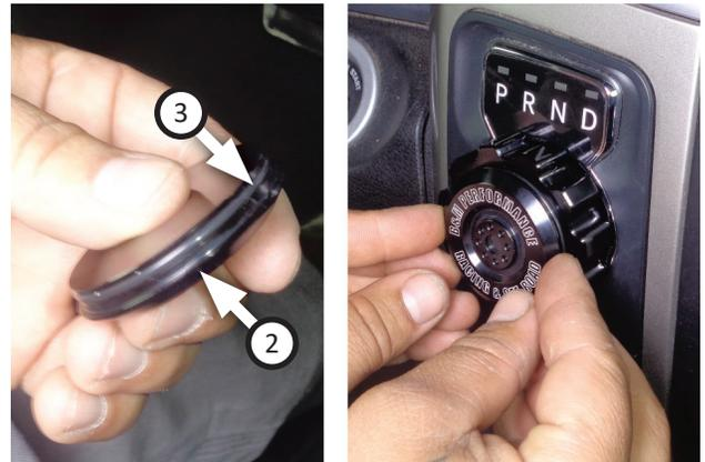
NOTE: Applying lubricant to O-ring will ease insert installation onto shifter knob.
