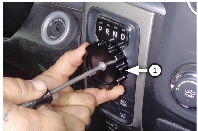
4. Set shifter knob (1) onto dial stem then fasten using screw (removed step 3).
