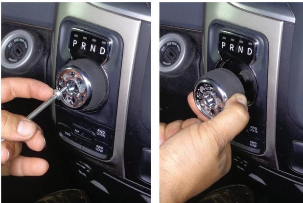
3. Remove screw from shifter knob then remove shifter knob from dial stem.
